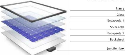
NEW BACKSHEET COATINGS OFFER THE FUNCTIONALITY OF CURRENTLY USED MULTILAYER FILM TECHNOLOGY, WHILE PROVIDING THE SAME LEVEL OF PERFORMANCE AND REVOLUTIONIZING THE PROCESS EFFICIENCY OF BACKSHEET PRODUCERS.
